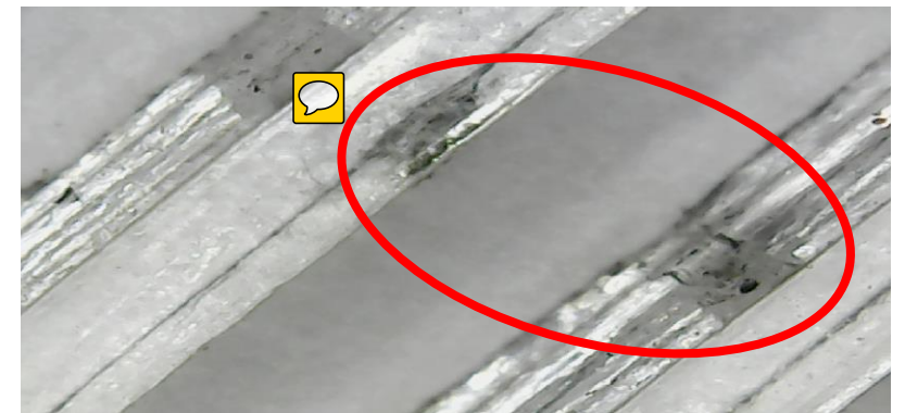
40 X Microscopic Image of dowel pin/elastic beam contact
